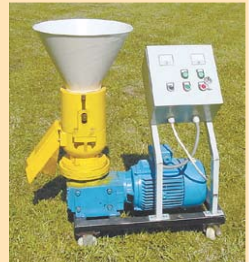
Pellets shown above were made by Tiger Tec's 7 1/2 hp. pellet mill (right). It's geared down to run slower and has more torque than other similar-size pelletizers.
