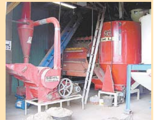
The Siedschlags recently set up a farm-sized pellet plant in their shop which includes a tub grinder, hammer mill, screener, and self-unloading wagons. Their goal is to automatically make 800 to 1,000 lbs. of pellets per hour.
